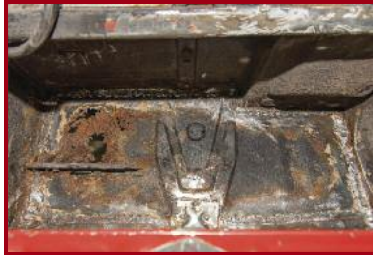
Once the car is raised on jacks, the battery box rust damage is more than obvious.
