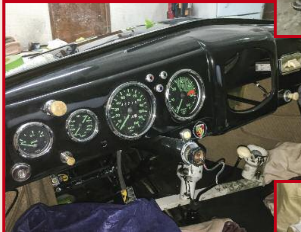
The unmistakable "pre-A" dash with its Störk "oel" combination gauge during the car's restoration.
