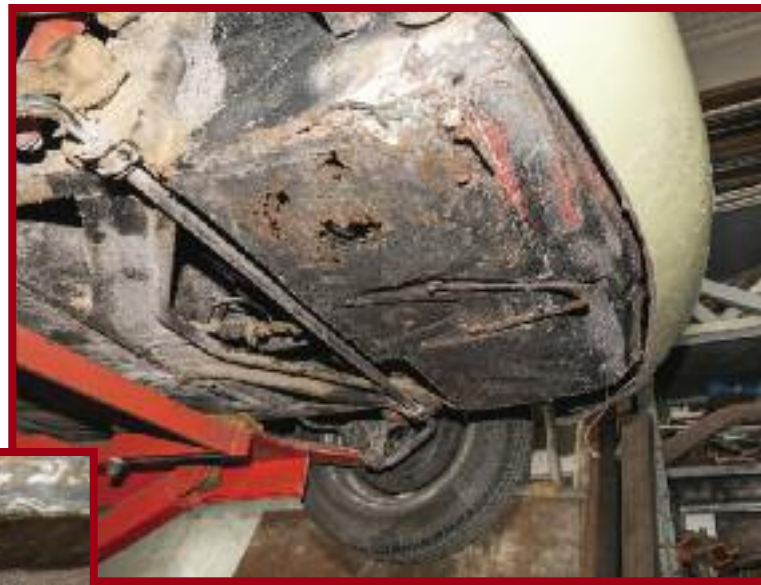
Once the car is raised on jacks, the battery box rust damage is more than obvious.
