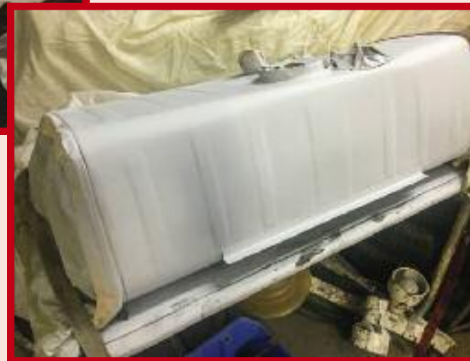
Primed and checked for leaks, the fuel tank awaits paint.
